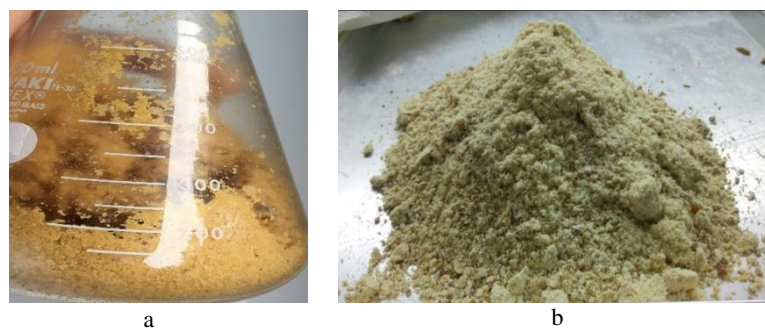
Figure 3. Wet (a) and dried (b) inoculum of Rhizopus oligosporus
